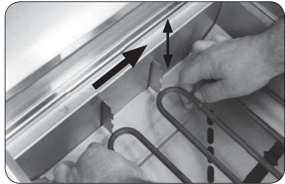
Fig. 14-1 Adjust cooking element
