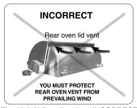
Fig. 12-3 Airflow direction - INCORRECT
