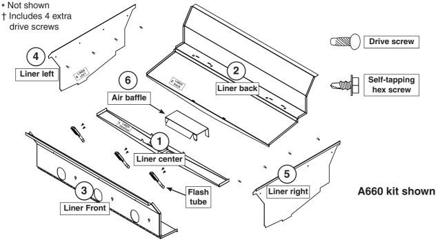
This firebox liner kit is for installation on Aurora grills with spark ignition only. Installation on an A660 is depicted in this instruction.
