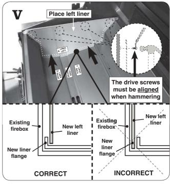
Place the left liner (item 4) as shown above. Rest the liner <a href="OVER">OVER</a> the front and rear liner flanges (hiding the flanges) and ensure the 4 holes are aligned with the 4 grill wall rivets. To secure the liner, align each drive screw (included in kit) with the corresponding hole and carefully hammer each drive screw into the panel. Use needle-nose pliers to assist in holding the drive screws properly.
