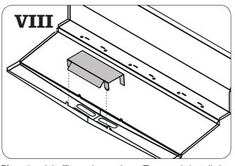
Place the air baffle as shown above. To properly install, the tabs must slide into the slots located on the liners.
