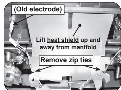
Fig. 2-5 Remove heat shield
