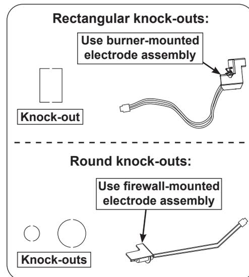
Fig. 3-5 Electrode assembly Identification
