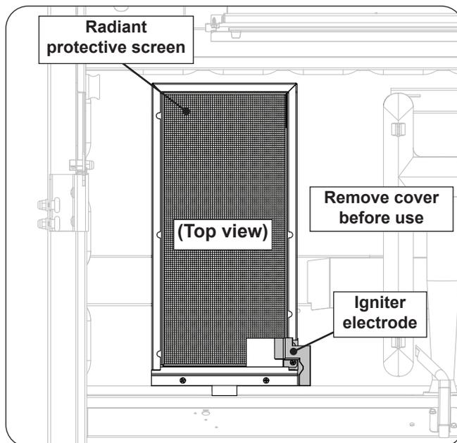
Fig. 8-1 Infrared burner overview
